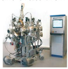
The Cryofox UHV Cluster System is a family of compact cluster tools, specific developed for PVD and PECVD processes in UHV environment. The systems are optimized in the mechanical design and control system for highest output of top quality research samples and process data. Major application fields are:
